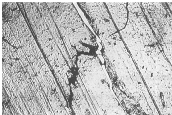
FIGURE 2 Microphotographs of transverse and longitudinal microcracks in PP, oxidized under stretching stress; PP-1, uninhibited sample; 130°C, air, \sigma = 10 MPa, \tau = 100 min.
